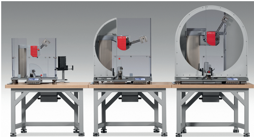
Pendulum impact testers are used, e.g., for assessing the deformation of the plastic even at high velocities. © ZwickRoell
